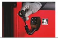
The integrated HF charger allows for quick and easy charging. The non-maintenance battery plugs directly into the mains.
