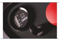
An battery indicator allows the operator to control the level of the load.
