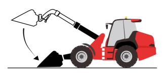
3 - Automatic «Return to Load": to easily return to a position (attachment and boom) predetermined by the operator. This function is particularly useful for loading operations.
