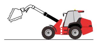
2 - **«Bucket Shaker»**: quickly empties the bucket without requiring the operator to make repetitive movements. Manure will not stay stuck to the bottom of the bucket.
