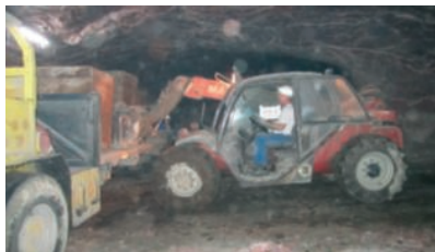
MVT 628 + rotating carriage + 1,200mm (47") forks
