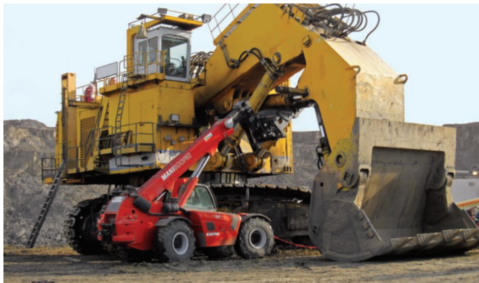
MHT 10160 + CH10 servicing a 9,80 ton (21605lbs) excavator
