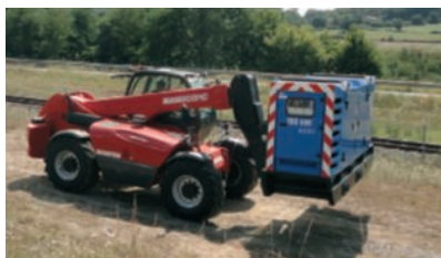
MHT 780 + TFF 2500 + 1,200mm (47") forks (handling a 100kW generator)
