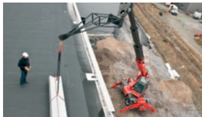
MRT 1840 with fixed Jib P 1200 remote controlled
