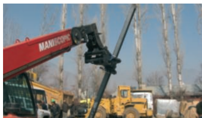
MT 1235 ST Handling HEB 120 Beam
