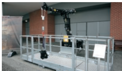
ORH 3.25-4m ARG 1,000kg (2200lbs) basket with 350kg (772lbs) Jib winch
