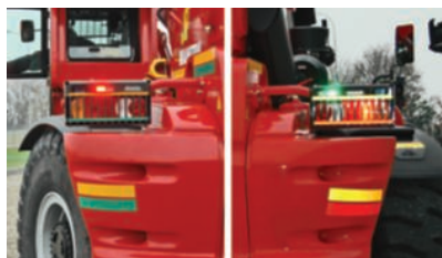
Signal lights for machine approach or withdrawal
