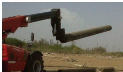
MHT 10210 handling a 12m (470"), 2,200kg (4850lbs) pipe with a prong
