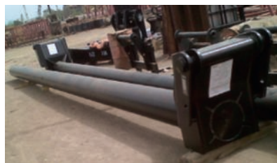
MHT 10225 with 7.5m (300"), 2t (4400lbs) spike
