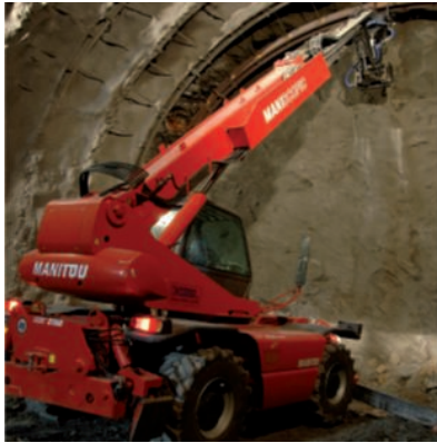
MRT 2150 with 4t (8820lbs) capacity Rib Erector
