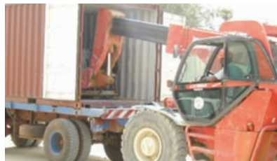
MHT 10180 with 3.5m (100"), 3t (6614lbs) capacity prong
