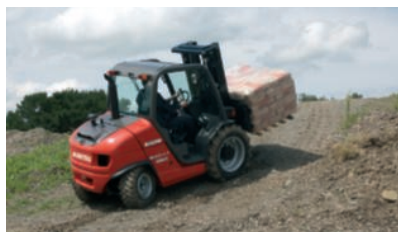
MH25-4 with side shifting carriage
