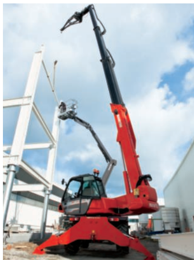
MRT 1840 with Jib winch PT 1200 remote controlled
