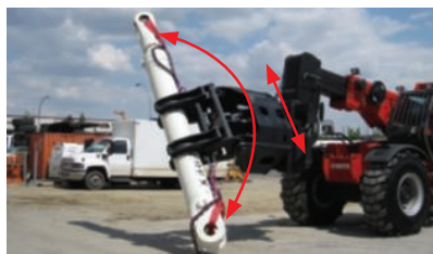
CH10 with movements (side shift + body rotation)
