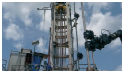
Rotate and place rod under the drilling head, continuous rotation clamp
