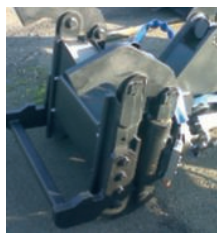
Rib Erector 2000kg (4400lbs) capacity clamping head
