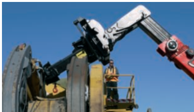
Titling cylinder change CH4 remote controlled
