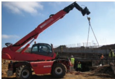
MRT 2150 with 5t (11020lbs) capacity winch
