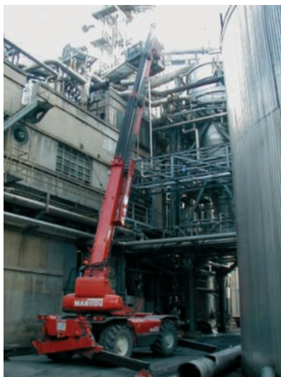
MRT 2150 with Jib winch 350kg (772lbs) mounted on man basket
