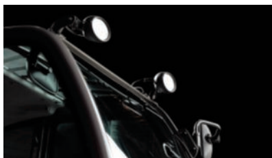
Working lights (front and back) located high on the cab
