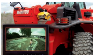
Smart pedestrian detection camera/screen
