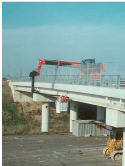
MRT 1840 + Aerial Jib, 2 negative position for bridge inspection
