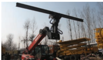
MT 1235 ST Handling HEB 120 Beam
