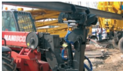
MT-X 1235 + rib erector 2t (4400lbs) + HEB 120 beam
