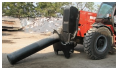
MHT 10180 with 10t (22046lbs) capacity spike
