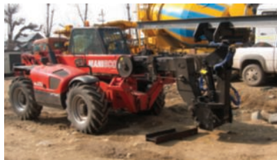
MT 1235 ST with Rib Erector 2000kg (4400lbs) capacity
