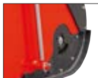
Left side distribution hydraulically controlled
