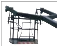
Pendular platform allows work under-bridges
