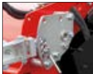
Interchangeable side brush (left or right)
